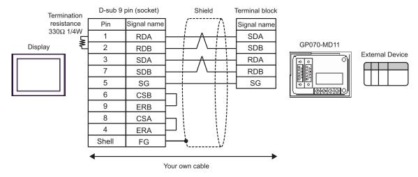
C) When using online adapter (CA4-ADPONL-01), 2-port adapter cable for AGP (CA3-MDCB11) by Pro-face and 2-port adapter II (GP070-MD11) by Pro-face.
