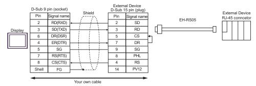
D. When using your own cable 2 and the conversion cable (EH-RS05) by Hitachi IES Co., Ltd.
