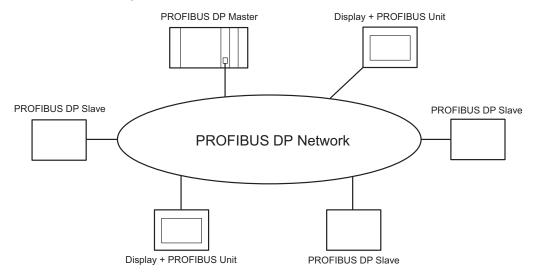
The I/O memory size of the PROFIBUS DP Master specifies maximum number of the Display which can connect to the PROFIBUS DP Master.
