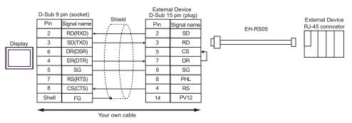
D. When using your own cable 2 and the conversion cable (EH-RS05) by Hitachi IES Co., Ltd.
