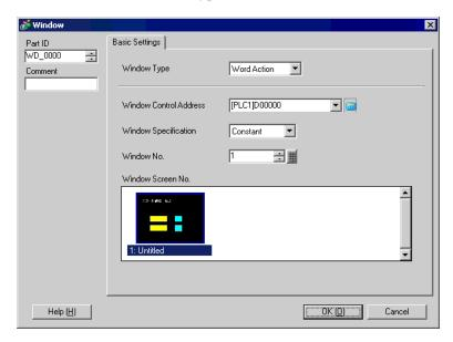
3 Set the word address (D100) which will control the window's display in [Window Control Address].
