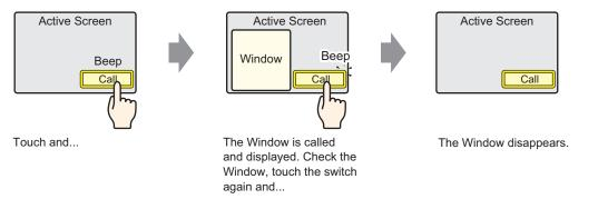
• As well as using a switch to display a window, a designated address in the device/PLC can also be used to turn a window's display ON/OFF.
