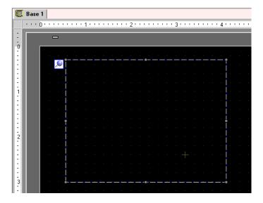
2 Double-click the placed Window part and the settings dialog box opens. Select [Activate Switch] from [Window Type].
