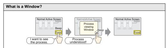
Screens that are not commonly used can be saved as Window Screens, and then displayed and hidden with a call button. They are suitable for temporary reference screens or error screens.
