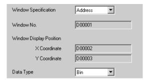
5 Click [OK]. The displayed Window Screen is now set up to change according to the value stored in the address.
