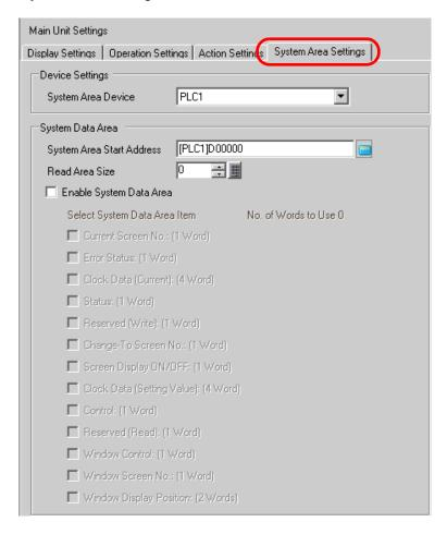
5 Set the device that will use the system area in [System Area Device], and set the allotted top address (D100) in [System Area Start Address].
