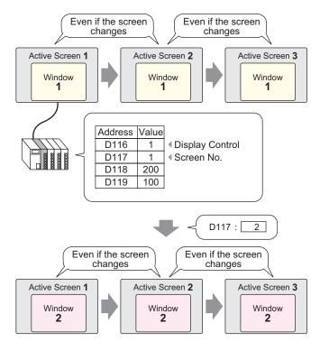
1 Select the [Project (F)] menu - [System Settings (C)] option - [Main Unit Settings] command, or click on the system settings window's [Main Unit Settings], and select the [Action Settings] tab.
