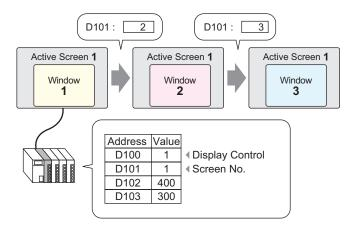
Multiple Window Screens can be changed and displayed to the specified screen.
