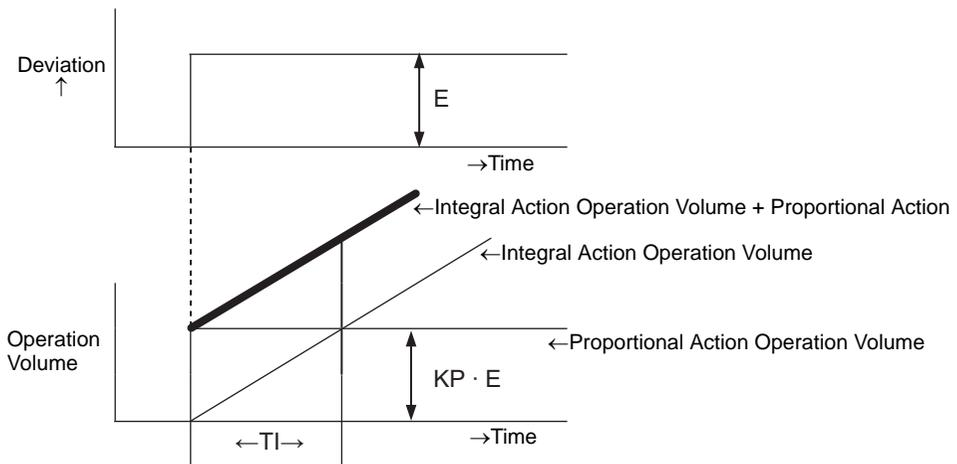
Uses the integral action as “PI action” combined with the proportional action, or as “PID action” combined with the proportional action and derivative action.” Integral action alone cannot be used.
