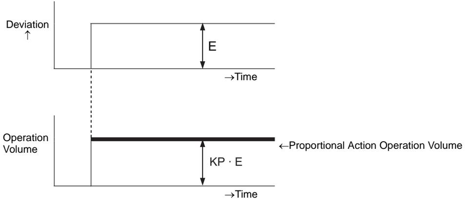
The operation volume varies in the range of 0 to 4095 (initial value). As KP increases, the operation volume proportionate to the deviation increases and the correcting action strengthens and causes offset (residual deviation).
