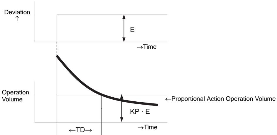
Uses the derivative action as “PD action” combined with the proportional action, or as “PID action” combined with the proportional action and integral action. Derivative action alone cannot be used.
