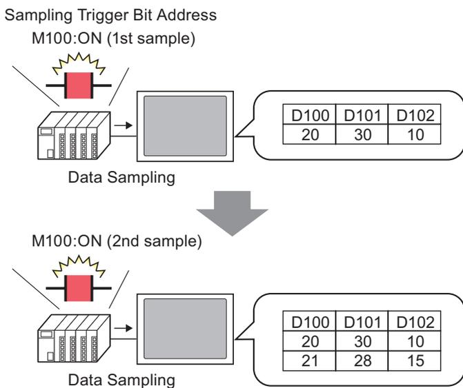
Sample data from the designated No. of Times, and set whether to automatically overwrite the oldest data and store the new data the next time the designated bit turns ON, or to stop sampling.
