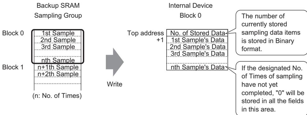
When storing sampling data to the internal device, the sampling round that is currently proceeding (which data has been stored) is saved in the top address in Binary format. For example, if the No. of Times is 5, and the current sampling round is 2, then [No. of Stored Data] will be "2". At that time, "0" will be stored in sampling data storage area for sample 3 and later.
