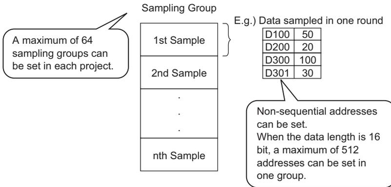
The sampled data can be displayed on the GP screen in group units, and saved to the CF-card.
