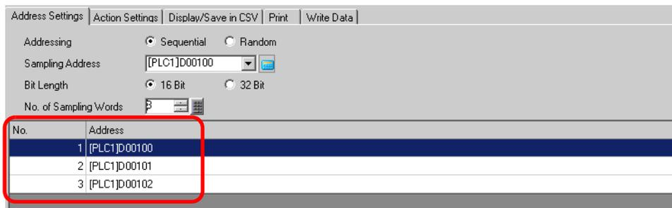
5 Open the [Action Settings] tab, and select [Execution Condition] as [Bit ON].
