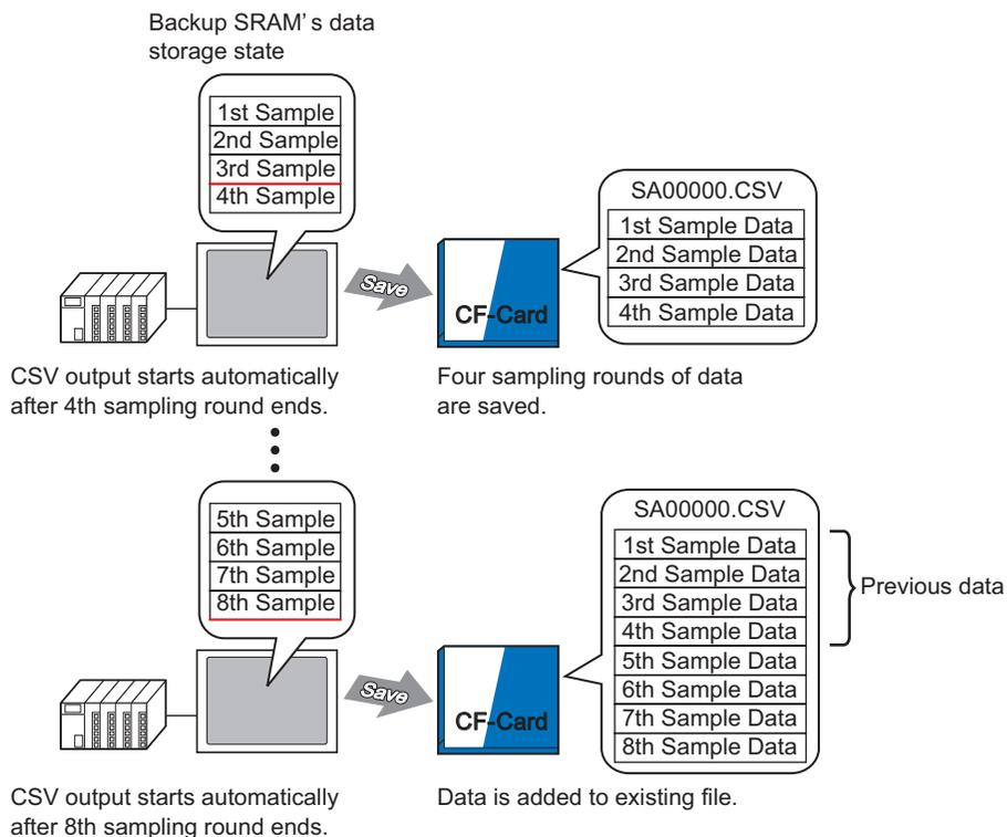
When auto save mode ends, even if there are contents still on the way to the GP (when the current sampling cycle has not completed), sampling data from up to that point will be written to the CF-card.
