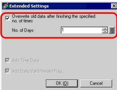
For the picture to the left, one day's data will be maintained in the GP. On the following day at the Start Time (8 a.m.), the previous day's sampling data will be overwritten in order and new data stored. If you do not want data to be overwritten, clear the [Overwrite old data after finishing the specified no. of times] check box. On the following day at the Start Time, sampling will not occur.
