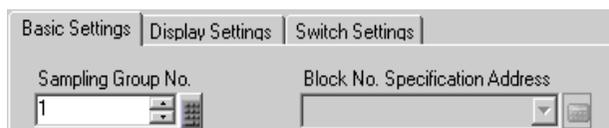
**NOTE** • When displaying a sampling group that does not have [Overwrite old data after finishing the specified no. of times] set in [Sampling Settings] - [Action Settings] tab - Advanced Settings, you must set a [Block No. Specification Address] in order to designate the blocks to display.
