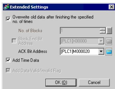
In the picture to the left, when data for the designated number of times (Example: 4) is stored to the GP and the trigger bit (M100) turns ON for the 5th time, data will be overwritten and stored starting from the 1st time's data.
