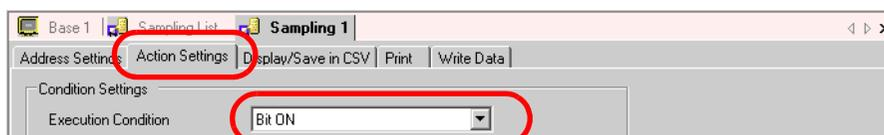
6 In [Sampling Trigger Bit Address], set the bit address (e.g.: M100) to control the data sampling operation. The data sampling will execute every time this bit turns ON.
