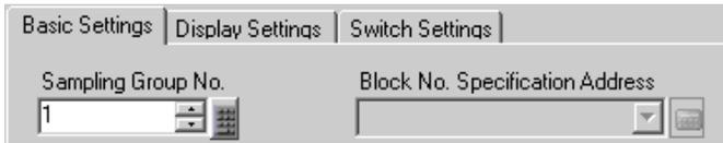
**NOTE** • When displaying a sampling group that does not have [Overwrite old data after finishing the specified no. of times] set in the [Sampling Settings] - [Action Settings] tab - Advanced Settings, you must set the [Block No. Specification Address].
