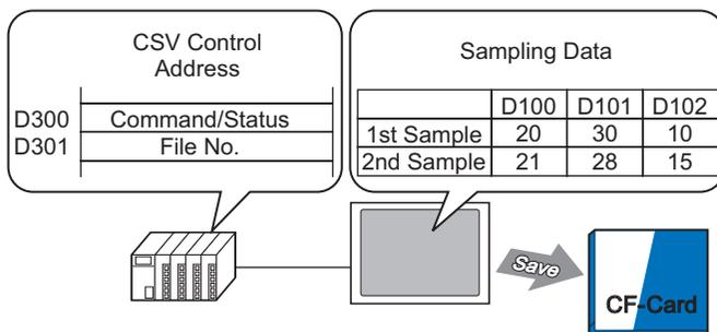
Store the File No. in the designated Control Address + 1, write a command to the Control Address and...
