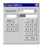
6 Click and select the [Device/PLC] and [Device]. Input an address from the keypad.(e.g.M100)
