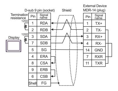
C) When using the online adapter (CA4-ADPONL-01), the connector terminal block conversion adapter (CA3-ADPTRM-01) by Pro-face and your own cable
