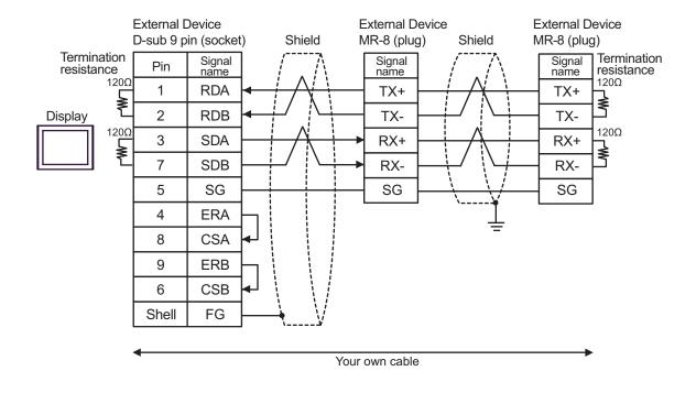
NOTE • When the External device has a SG terminal, connect it to the SG terminal of the Display.
