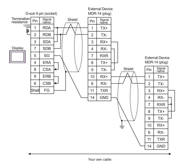
C) When using the online adapter (CA4-ADPONL-01), the connector terminal block conversion adapter (CA3-ADPTRM-01) by Pro-face and your own cable
