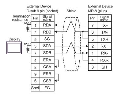
C) When using the online adapter (CA4-ADPONL-01), the connector terminal block conversion adapter (CA3-ADPTRM-01) by Pro-face and your own cable
