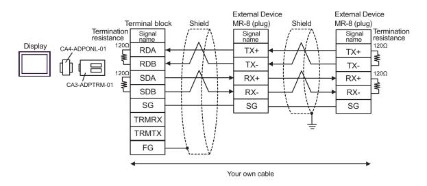
• When the External device has a SG terminal, connect it to the SG terminal of the Display.
