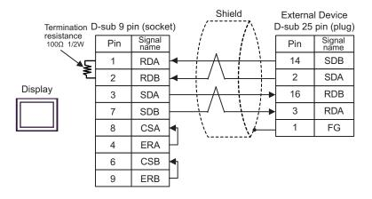
C) When using the online adapter (CA4-ADPONL-01), the connector terminal block conversion adapter (CA3-ADPTRM-01) by Pro-face and your own cable
