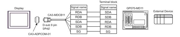
B) When using your own cable and 2-port adapter II (GP070-MD11) by Pro-face.
