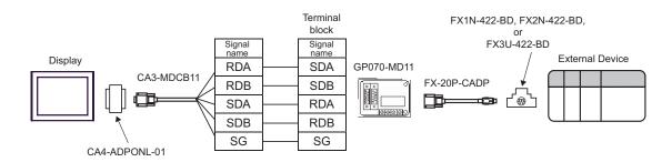
D) When using the online adapter (CA4-ADPONL-01) by Pro-face, your own cable, the 2-port adapter II (GP070-MD11) by Pro-face, the connector conversion cable (FX-20P-CADP) by Mitsubishi Electric Corp. and the function extension board (FX1N-422-BD, FX2N-422-BD or FX3U-422-BD) by Mitsubishi Electric Corp.
