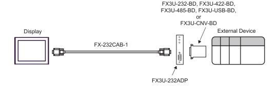
B) When using your own cable, the communication adapter (FX3U-232ADP) by Mitsubishi Electric Corp. and the function extension board (FX3U-232-BD, FX3U-422-BD, FX3U-485-BD, FX3U-USB-BD or FX3U-CNV-BD) by Mitsubishi Electric Corp.
