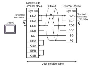
\*1 The resistance in the Display is used as the termination resistance. Set the value of the DIP Switch on the rear of the Display as shown in the table below.
