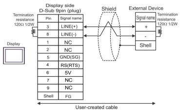
• The 5V output (Pin #6) on the Display is the power for the Siemens AG's PROFIBUS connector. Do not use it for other devices.
