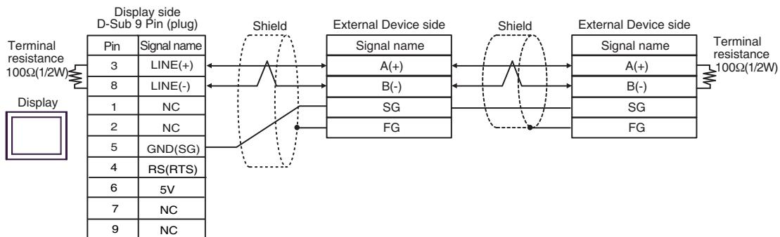
**IMPORTANT** • The 5V output (Pin #6) on the Display is the power for the Siemens AG's PROFIBUS connector. Do not use it for other devices.
