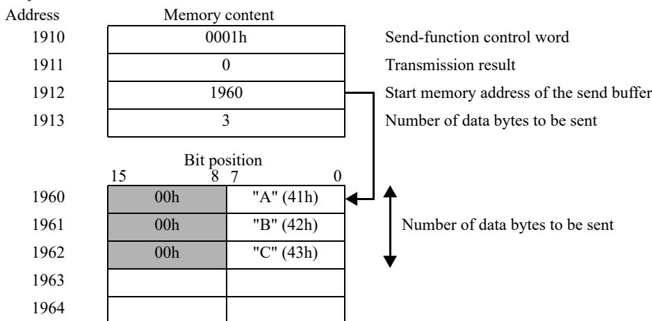
\* Be sure to store the data to be sent per byte in the lower bytes of each address in the memory table (word: 16-bit length).
