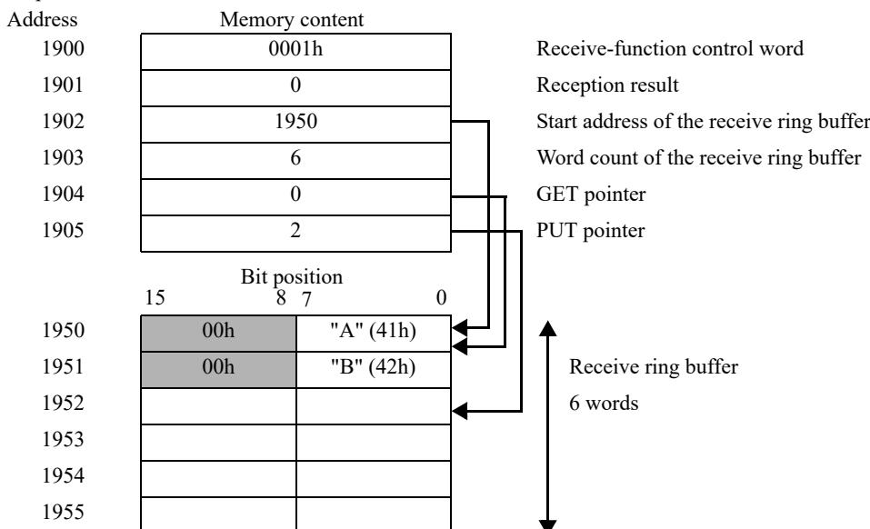
Received data is stored per byte in the lower bytes of each address in the memory table (word: 16-bit length).
