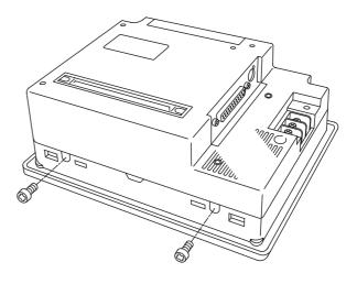
3) Pull the unit's Rear Cover straight up to remove it.
