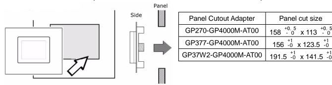
Fix the back side of the panel with the fasteners.
