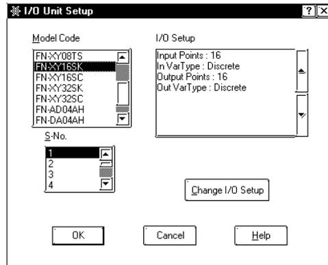
3. Change the “Model Code” field’s “FN-XY16TS” to “FN-XY16SK.”
