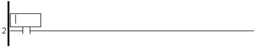
The instruction now appears on the selected rung. Also, there is a box above it with a flashing cursor inside. This is the “Instruction Parameter Box,” where you enter a variable to associate with the instruction. This will be explained in more detail later in this chapter.
