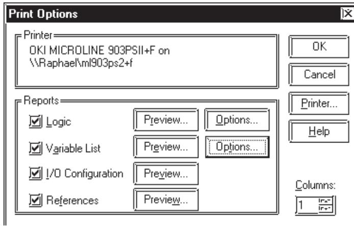
You can select the number of columns (1 to 4) into which your report will be formatted. In the [**Reports**] area, there are four checkboxes labelled [**Logic**], [**Variable List**], [**I/O Configuration**] and [**References**]. These checkboxes provide the following options when printing out ladder logic program data.
