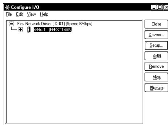
6. Up to 63 units (when two lines are used) can be connected with the Flex Network driver. Use the same method for selecting a module for another unit.
