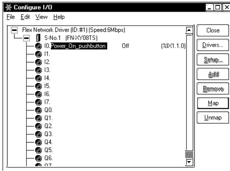
The 'Power\_On\_pushbutton' variable (NO variable) on rung 3 now has a series of digits and letters above it. This is the IEC I/O address of that variable.
