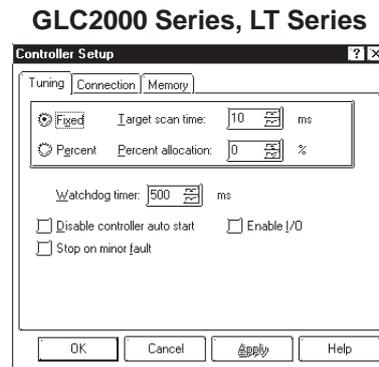
When you set parameters on the [Tuning] tab, you are setting the parameters the ladder logic program uses when it is written to the GLC Controller. Subsequently, whenever this particular program is run, the GLC Controller will use these settings, unless they are changed manually. These settings are unique to this program.
