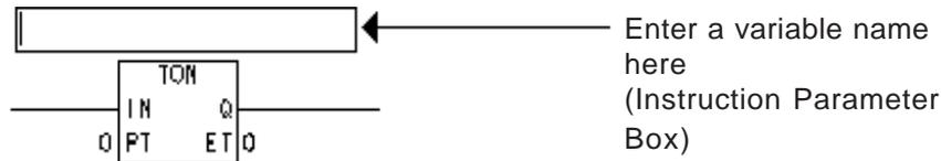
3. Double-click the area immediately to the left of the PT element in the TON instruction. The [Data Value] dialog box opens. Here, enter the preset time in milliseconds that will elapse before output (Q) is turned ON. (Assigning variables and other operands to instructions will be discussed in the next section.)
