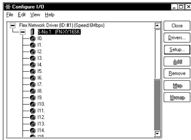
Displayed below ‘S-No.1 (FN-XY16SK)’ are 16 input terminals and 16 output terminals associated with the Flex Network module displayed. You will assign variables to them later in this tutorial.
