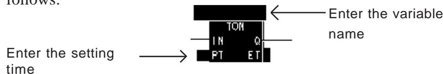
Above the TON instruction a black highlighted area will appear. This is where you enter the variable to be assigned to the TON instruction. Next to the Preset (PT) element is another black highlighted area. This is where you enter the preset time in milliseconds.
