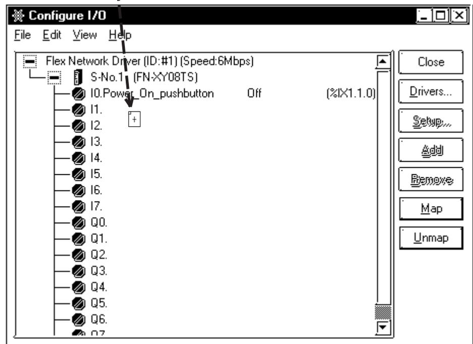
**When you assign (click and drag) a variable to [Configure I/O] from the [Variable List] or [Description List] window, that I/O attribute is enabled and any other variable attribute will be changed to Input/Output.**
