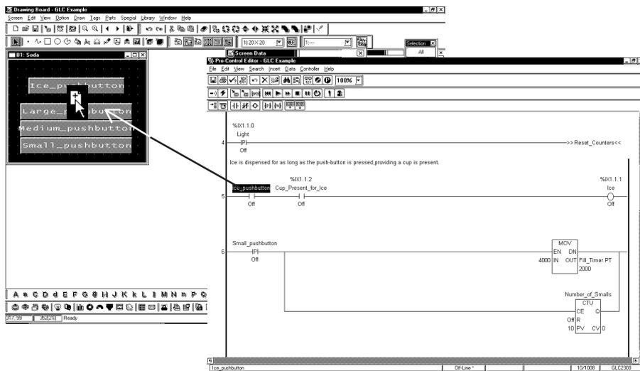
2. Drop the button on the Screen Editor. The “Select Parts” dialog box will appear on the screen. Select “Bit Switch,” then click [OK].
