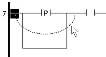
When the mouse button is released, a new branch will be inserted over the previous branch.
