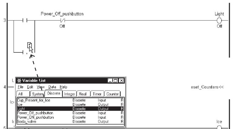
The variable is then assigned when the cursor is released. As long as the cursor appears as a
