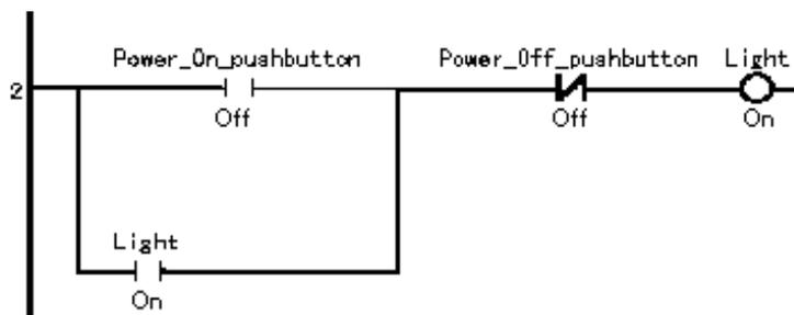
3. Right-click the ‘Light’ variable assigned to the output coil on rung 2.
