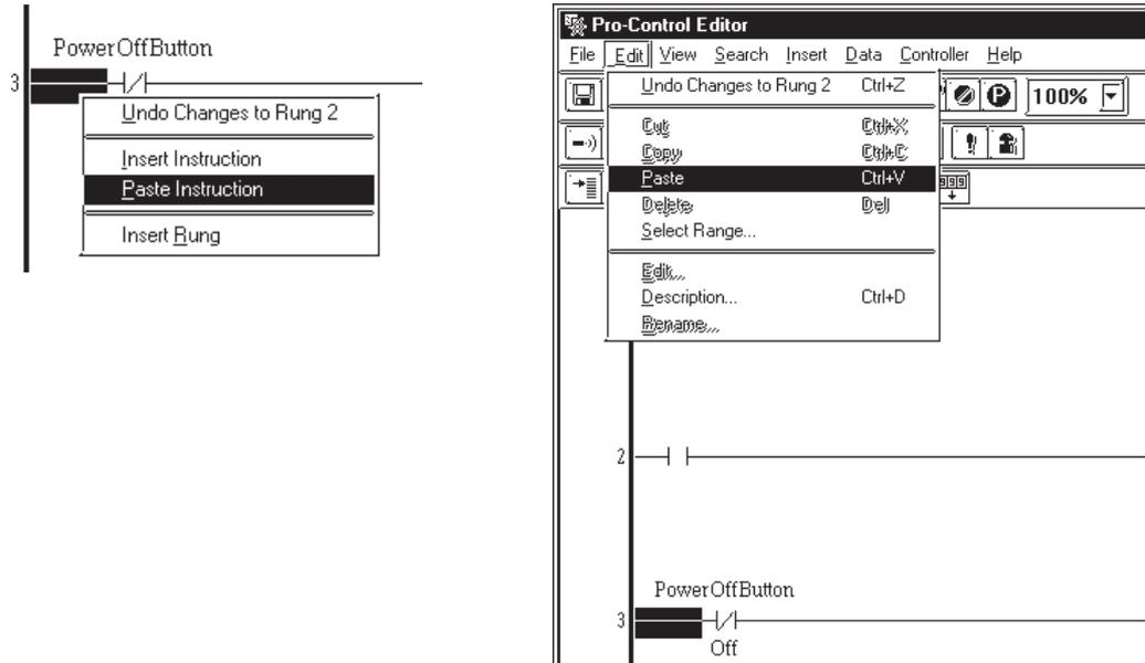
3. The copied instruction is now pasted (inserted) into the desired rung.
