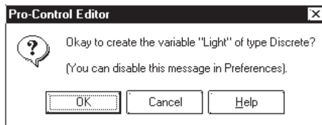
4. Click [OK]. In the [Variable List] dialog box, the “Light” variable appears in the list. The Editor has automatically assigned it a *variable type*. In this case it has assigned it as an internal discrete variable.
