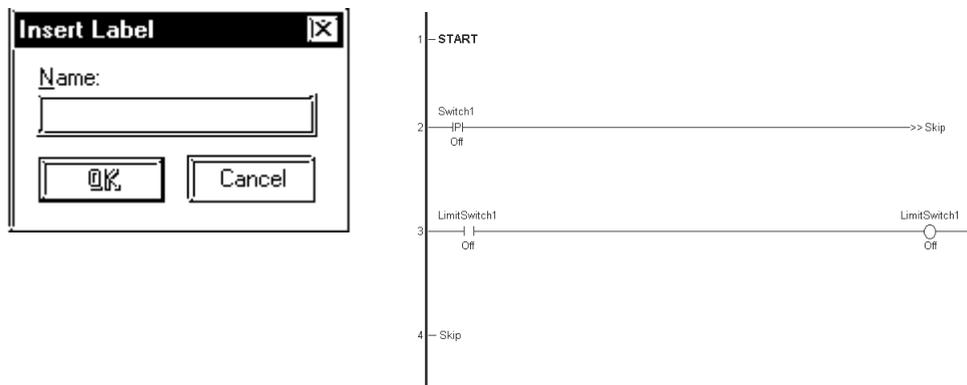
This is the name that is designated in the **[JMP]** instruction in your ladder logic program. The same rules that apply to the naming of variables also apply to the naming of labels.
