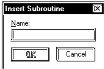
3. Type "Reset\_Counters" in the [Name] field of the [Insert Subroutine] dialog box. A maximum of 32 text characters, numbers, or underscore characters can be used for a subroutine name. Variable names cannot begin with numerical characters and cannot contain spaces.
