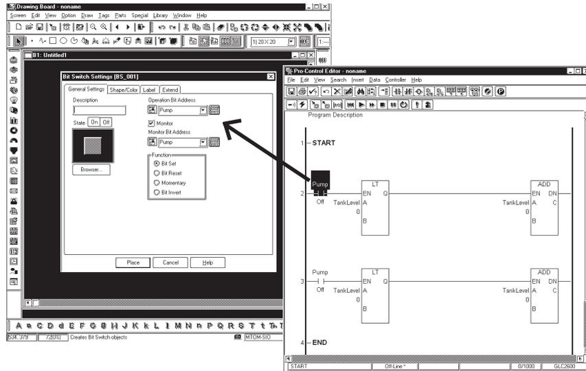
5. Set the “**Operation Bit Address**” to “**Pump**,” then click [Place]. The “**Pump**” Bit Switch is created in GP-PRO/PB III Editor.
