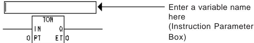
3. Double-click the area immediately to the left of the PT element in the TON instruction. The [Data Value] dialog box opens. Here, enter the preset time in milliseconds that will elapse before output (Q) is turned ON. (Assigning variables and other operands to instructions will be discussed in the next section.)
