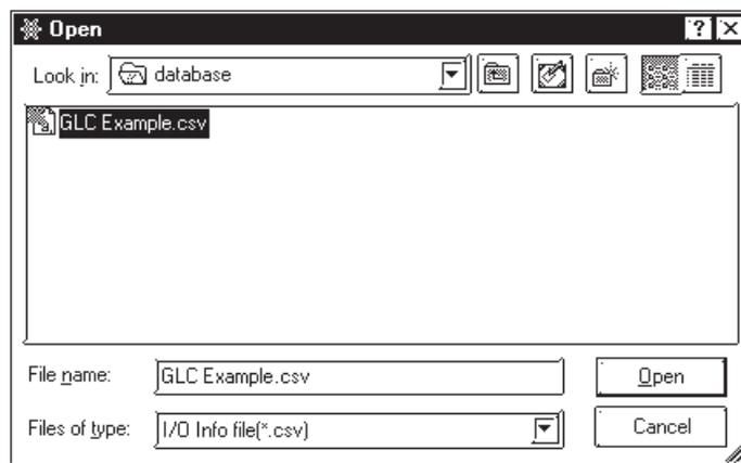
5. The CSV file's variables will be read in and allocated automatically to the Flex Network.
