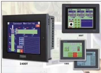
(counterclockwise from top): The 1510 Industrial PC is a node box that supports a remote monitor. The GLC2400T integrates information connectivity, OI, and I/O control. GP-PRO/PB III supports the latest GLC2000 series products with control logic developed using the Pro-Control v3.0 IEC 61131-3-compatible ladder logic editor.
