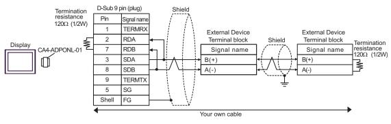
E) When using the COM port conversion adapter (CA3-ADPCOM-01) and the terminal block conversion adapter (CA3-ADPTRM-01) by Pro-face
