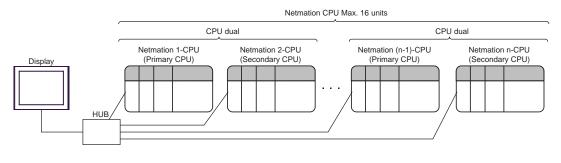
• 1:n Connection (Ethernet single/Netmation CPU single/dual mixed)
