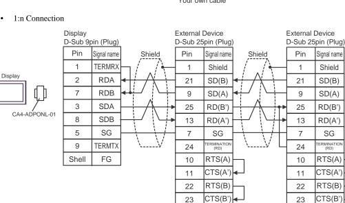
\*1: Notation of RD(A'), RD(B'), SD(A) and SD(B) are different by the external device.
