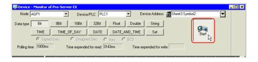
Device values are displayed according to the screen size with the specified device address (symbol) at the top.
