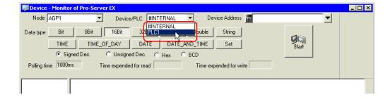
**5** Input directly the address of the monitoring device in [Device Address], or click the list button to select the symbol.
