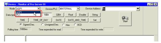
4 Click the list button of [Device/PLC] and select a Device/PLC having a monitoring device.
