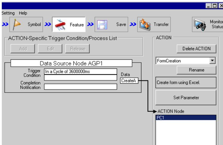
2 Select the trigger condition name "CreateAForm" from the tree display on the left of the screen.
