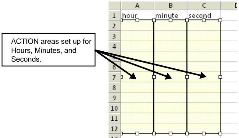
The above illustration shows ACTION areas that get the Hours, Minutes, and Seconds from the external device's clock register, and populate the data in columns A, B, and C. Columns A, B, and C each have different ACTION areas set up.
