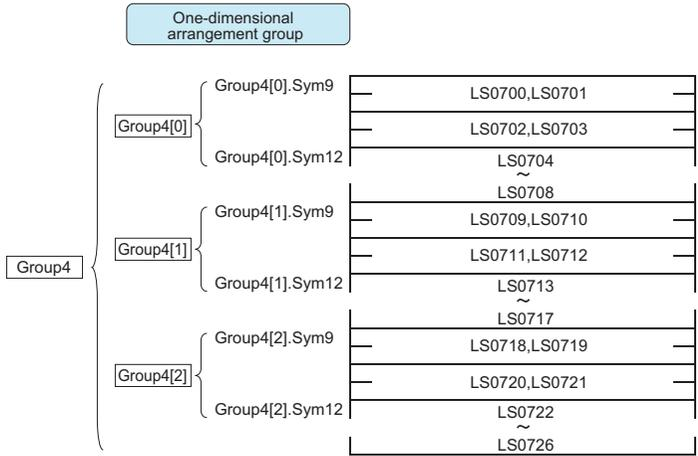
Note: Bit offset symbols (Sym10, Sym11) do not have the work for group access. However, they accept unit access. The works at that time are same as that for bit symbol.
