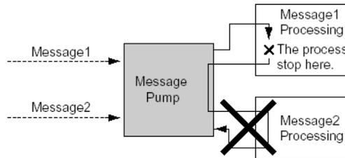
In such case, force the message pump to run. (calling DoEvents,VC for VB, or GetMessage() and DispatchMessage() for VC)
