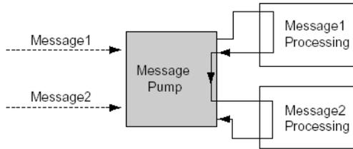
In this case, assume that it takes long time for processing message 1. Then the message pump cannot process message 2 without recovering.
