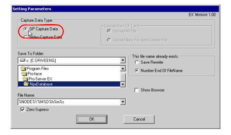
6 Set "Desktop" for [Save To Folder] as a folder to store the file to write data in, with the default file name "%NODE%Y%M%D%h%m%s".
