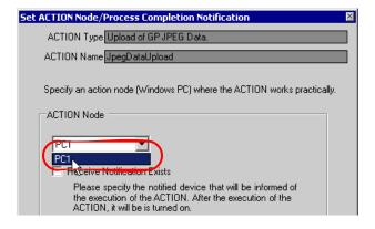
**3** Turn off the [Receive Notification Exists] check box, if checked.
