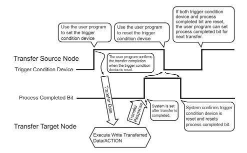
The following chart describes the summary of the rigger condition device, [Bit Showing Completion of the Process], [Bit Showing Processing Result (Success/Failure)], [Error Code Storage Location], [Abnormal Device IP Address Storage Location] and the timing to set the receipt notification device described later.
