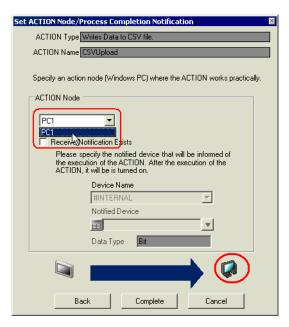
10 Turn off the check box of [Receive Notification Exists], if checked.
