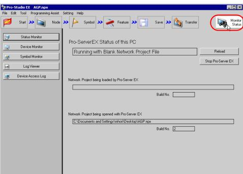
To perform device monitoring, 'Pro-Server EX' should be operating. When 'Pro-Server EX' is under suspension, click the [Reload] button to start the operation.
