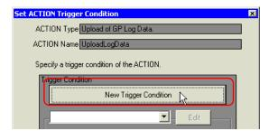
**3** Enter the trigger condition name "CollectAtConstantTimes" in [Trigger Condition Name], and select "AGP1" in [Node Name] as a name of the data transfer source.
