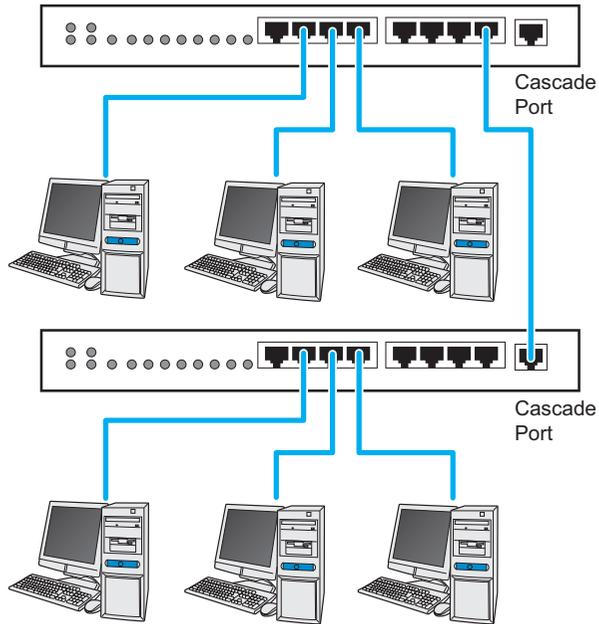
■ Ethernet Cable (10BASE-T/100BASE-T compatible UTP straight cable)
