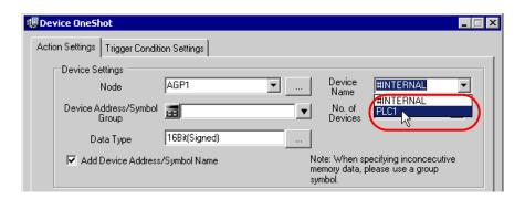
4) Click the list button of [Device Address/Symbol Group] and select "PLC1 data" as a symbol of the data to read out.
