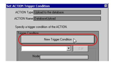
**3** Enter the trigger condition name "TurnOnReadStartBit" in [Trigger Condition Name], and select "AGP1" in [Node Name] which has the device to serve as the trigger condition (trigger).
