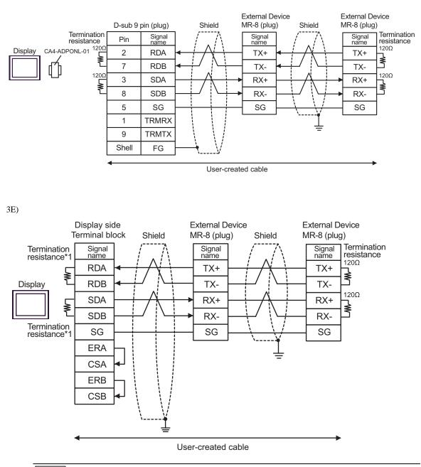
• When the External device has the SG terminal, connect it to the SG terminal of the Display.
