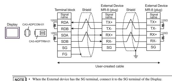
NOTE when the External device has the SO terminal, connect it to the SO terminal of the Disp
