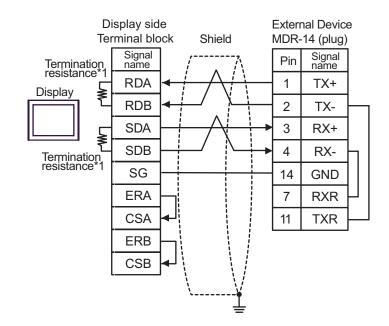
\*1 The resistance in the Display is used as the termination resistance. Set the value of the DIP Switch on the rear of the Display as shown in the table below.
