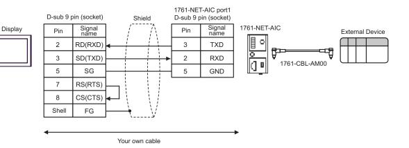
GP-Pro EX Device/PLC Connection Manual
