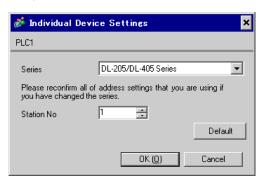
For communication settings, use the DIP switches on the CPU unit. To set the station No., use the instruction word programmer (S-01P). After completing the settings, reboot the External Device to enable them. Please refer to the manual of the External Device for details.
