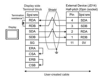
\*1 The resistance in the Display is used as the termination resistance. Set the value of the DIP Switch on the rear of the Display as shown in the table below.
