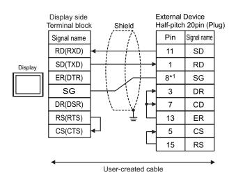
\*1 When connecting with 30i-Model A, 31i-Model A or 32i-Model A, The pin number of SG changes with ports to be used.
