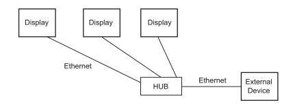
• The number of GP units has no limit. Note that more number of connecting units will result in increasing the communication load.
