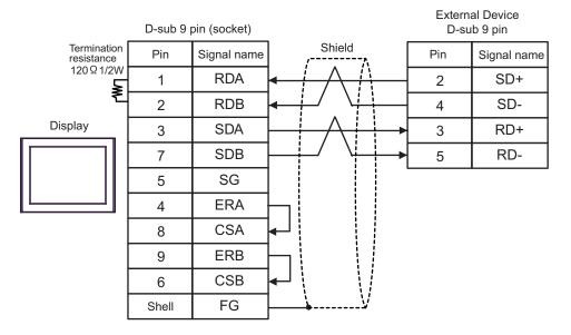
C) When using the online adapter (CA4-ADPONL-01), the terminal block conversion adapter (CA3-ADPTRM-01) by Pro-face and your own cable
