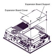
(3) Remove the four screws of the expansion board base, and then remove the board base. For PS-3651A Series, this step is unnecessary.
