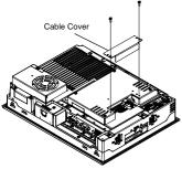
(5) Pull out the two connectors, Backup Output Connectors (CN2) and Control Signal Connector (CN3), as indicated below.
