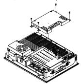
(7) Install a new battery unit in place. Return the cable cover and expansion board cover to their original positions on the PS-A unit by reversing steps (2) to (6) above. The tightening torque is 0.5 to 0.6 N•m.
