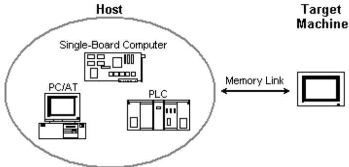
Communication between the host and target machine begins at the host. In other words, the host is the only one that can initiate communication. Even though an application exists on the target machine, and data values can change either through user inputs, scripts, or mapping to system variables, the target machine cannot initiate communications with the host.
