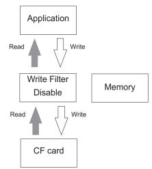
• Turning OFF the power at the time of writing into CF card leads to data damage. When using this unit, use it with the Write Filter effective. Prevention of writing into the CF card is expected to prevent being damaged or prevent the CF card life cycle (Reference: 0°C - 70°C, Writing/Delete Times: 300,000 times per block) from declining as well.
