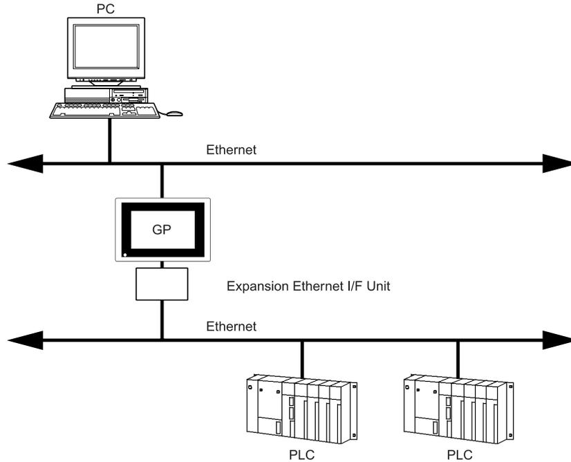
After attaching the Expansion Ethernet I/F Unit, your GP/GLC unit is now equipped with two Ethernet I/F units. (The Ethernet Expansion Unit cannot be used with the GP-2400 Series or GLC2400 Series units.)
