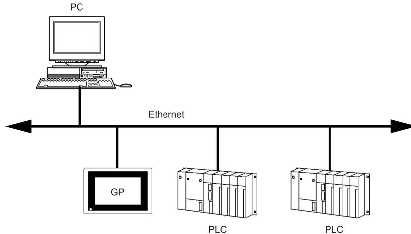
Using the GP/GLC's internal Ethernet I/F to communicate with a PLC allows you to also use the 2-Way Driver feature. However, while you will need only one IP Address, you will need to designate two Port No.s. One will be for when you transfer data to a PLC, and the other will be when using the 2-Way feature.
