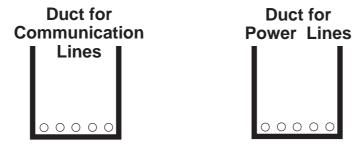
If the wires must be placed in the same duct, separate them via an earthed/grounded divider.
