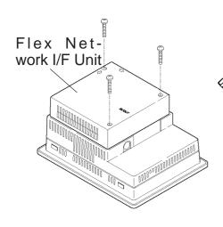
3) Attach the Flex Network unit and secure it in place with its three (3) attachment screws.
