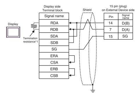
\*1 The resistance in the Display is used as the termination resistance. Set the value of the DIP Switch on the rear of the Display as shown in the table below.
