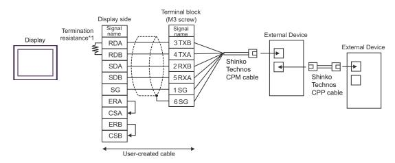
\*1 The resistance in the Display is used as the termination resistance. Set the value of the DIP Switch on the rear of the Display as shown in the table below.
