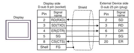
2B) Display side External Device side Terminal block D-sub 25 pin (plug) Shield Signal name Signal name Pin Display RD(RXD) 2 SD SD(TXD) 3 RD ER(DTR) 6 DR 7 SG SG CS(CTS) 20 ER
