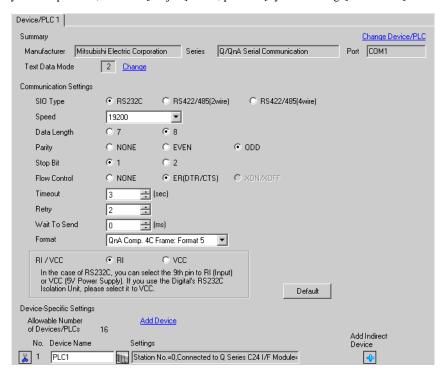
To display the [Individual Device Settings] dialog box, from [Device-Specific Settings] in the [Device/PLC] window, select the external device and click [Settings] .
