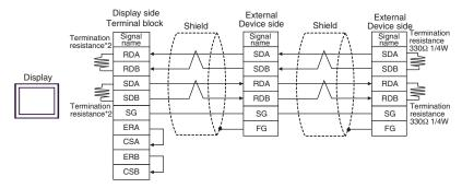
\*2 The resistance in the Display is used as the termination resistance. Set the value of the DIP Switch on the rear of the Display as shown in the table below.
