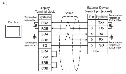
\*1 The resistance in the Display is used as the termination resistance. Set the value of the DIP Switch on the rear of the Display as shown in the table below.
