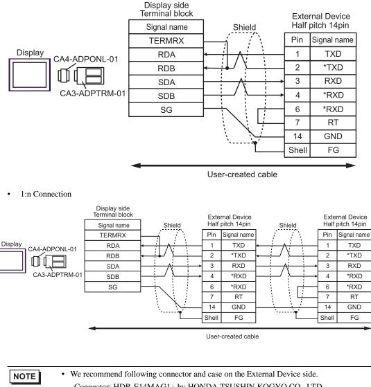
Connector: HDR-E14MAG1+ by HONDA TSUSHIN KOGYO CO., LTD. Case: HDR-E14LPA5 by HONDA TSUSHIN KOGYO CO., LTD.
