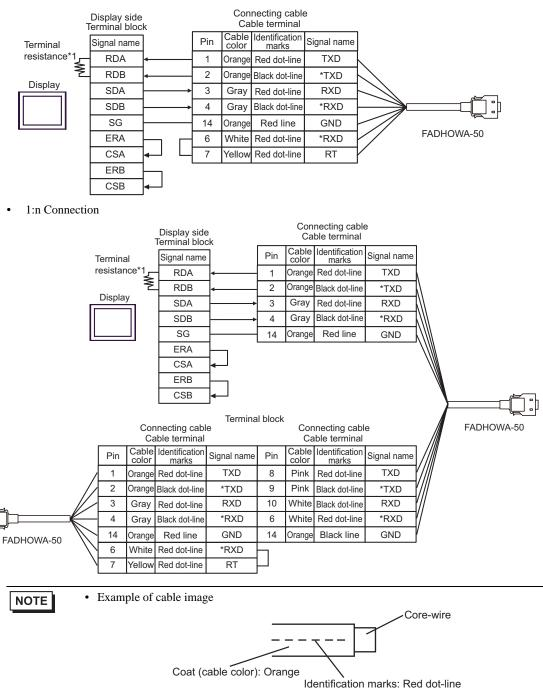
In the example above, the cable color is orange, and the identification mark shows red dotline, which means TXD.
