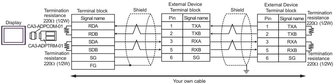
**NOTE** • When IPC is used as the Display, the terminal resistance of 220Ω can be inserted by the fact that the dip switch 5, 6 of IPC is turned to ON.
