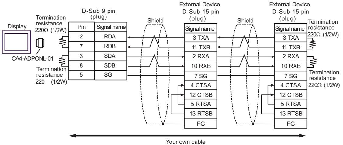
**NOTE** • We recommend CO-SPEV-SB(A)3P\*0.5 by Hitachi Cable, Ltd. for the connection cable.
