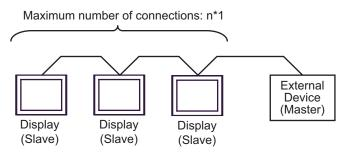
\*1 The number of Displays (Slaves) you can connect depends on the External Device. Check the specifications of the External Device.
